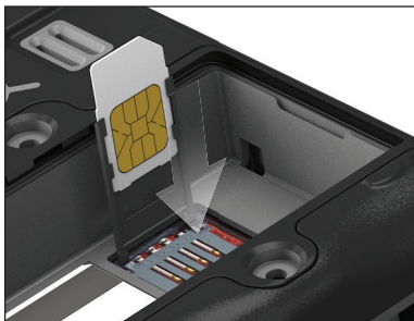
Inserting the SIM card
